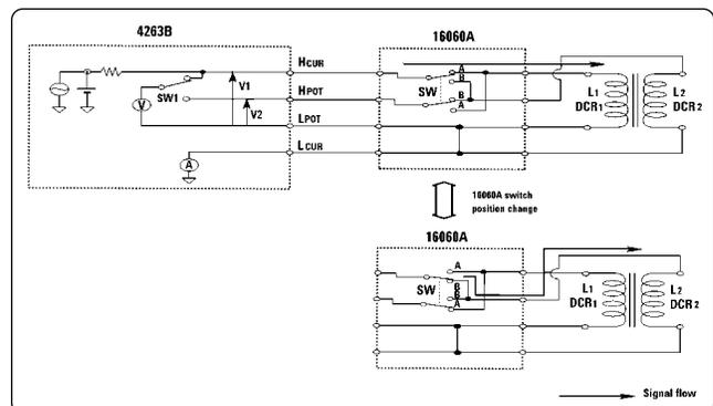
Figure 2. Agilent 16060A block diagram
