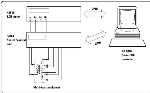
Figure 3. System configuration for multi-tap transformer
