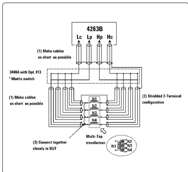
Figure 5. System construction
