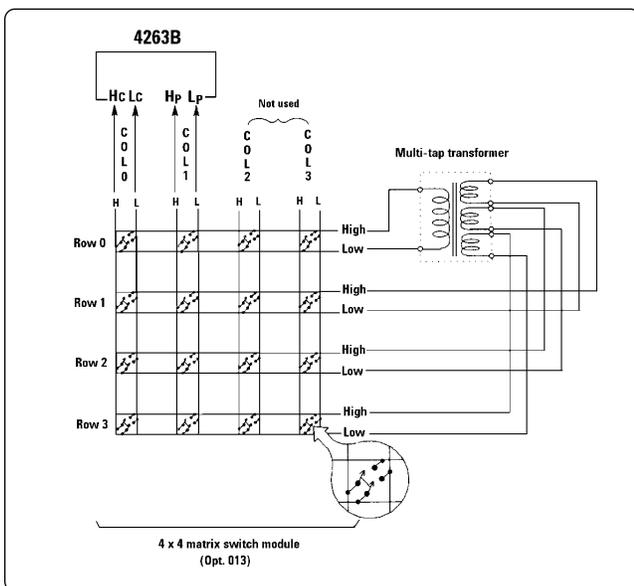
Figure 4. Option 013 4 x 4 matrix module
