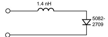
Figure 2A. Single Frequency Series Tuning, Impedance Coordinates.
