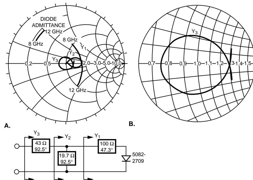
Figure 4. Three Element Mixer Matching Circuit, Admittance Coordinates.
