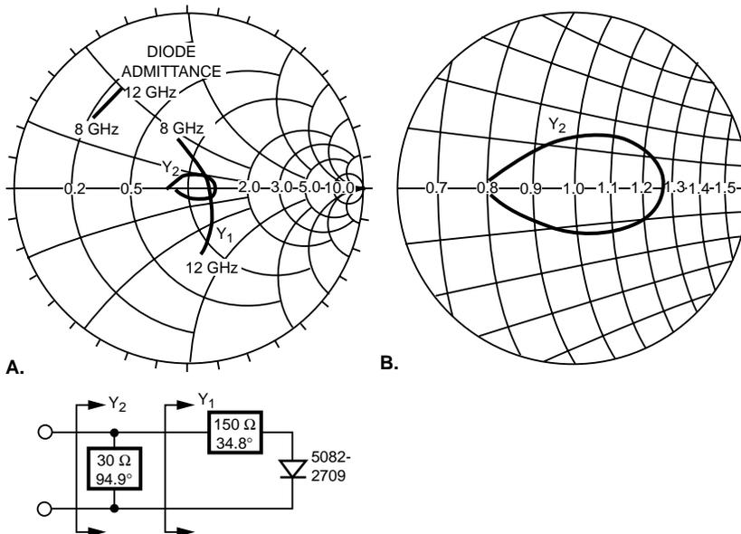
Figure 3. Two Element Mixer Matching Circuit, Admittance Coordinates.
