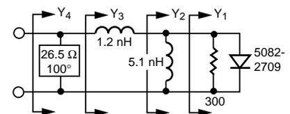
Figure 11. Detector Matching with Shunt Inductance, 50  $\mu$ A Bias, Admittance Coordinates.
