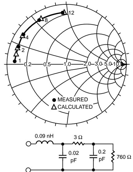
Figure 5. 5082-2709 Beam Lead Diode Admittance, 50  $\mu$ A Bias.
