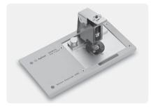
16197A bottom-electrode SMD test fixture
