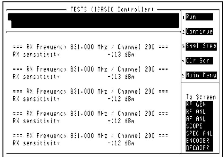
With the set-and-measure method, the user sets the RF level at which the test is performed and the measurement returns a “pass” if block error rate is better than 5%. The iterative test uses a binary search scheme to find the actual RF level at which the block error rate exceeds 5%.
