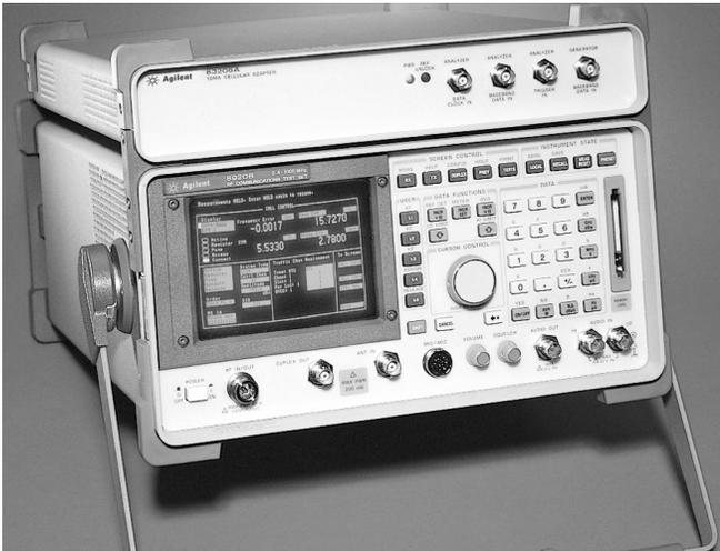
**The Agilent 8920B test set with the 83206A TDMA cellular adapter**
