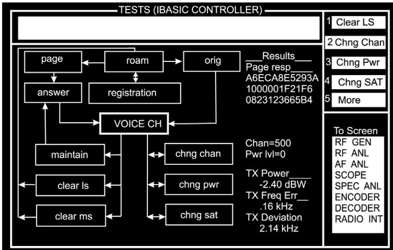
Using the on-screen flowchart program, you can troubleshoot a phone as it gains access to a system, and while on a voice or a digital traffic channel.
