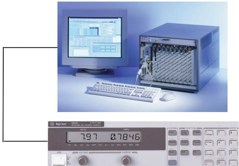
Figure 3: Setup with controller and GPIB power Supply
