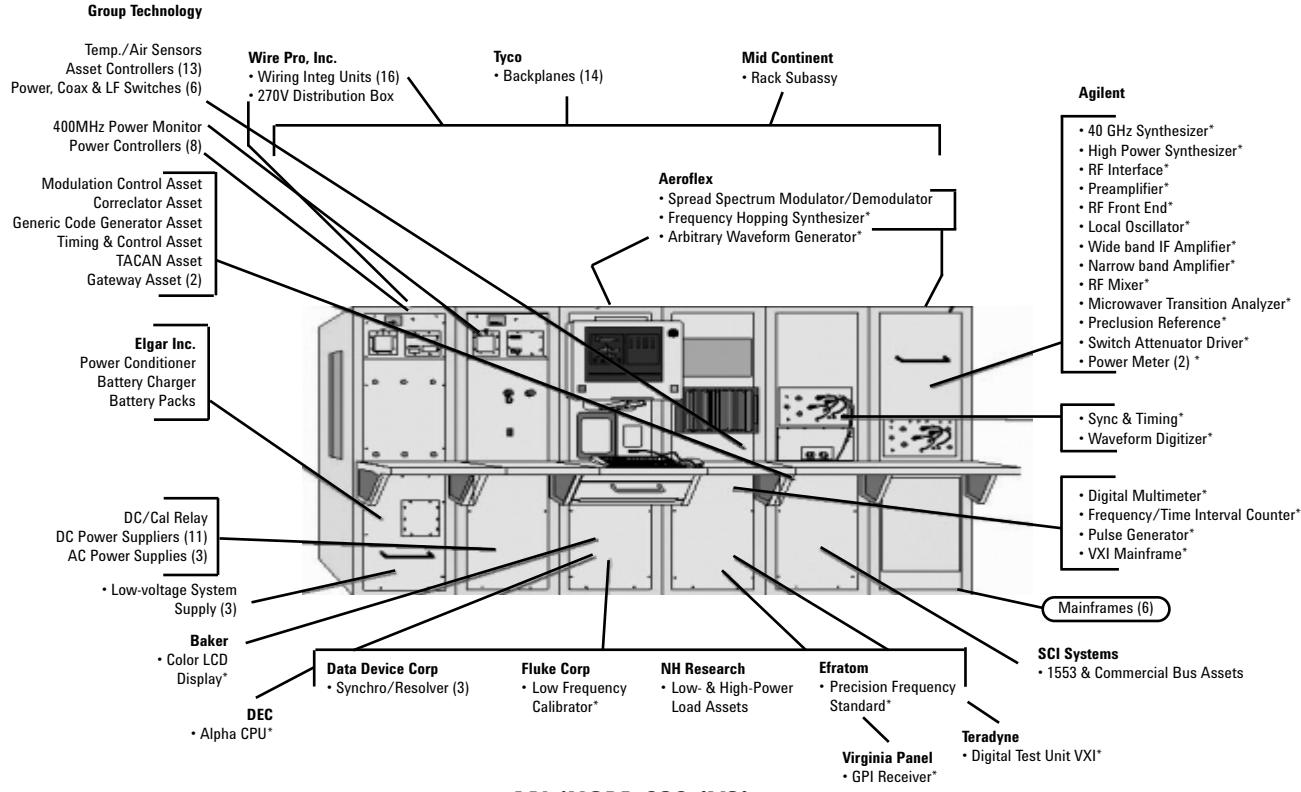
Figure 2: Block diagram of the CASS system
