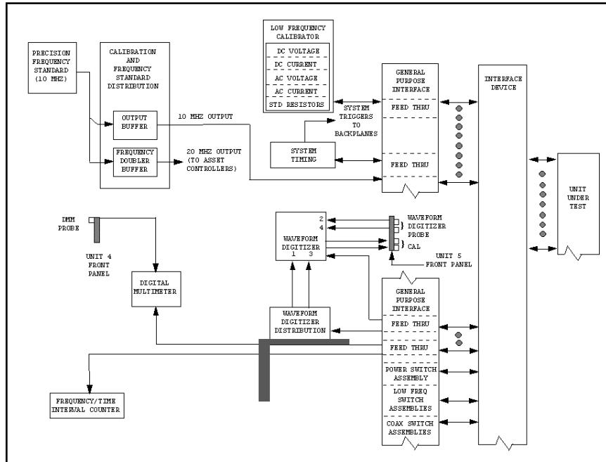
**Figure 3: Hybrid test station functional block diagram**
