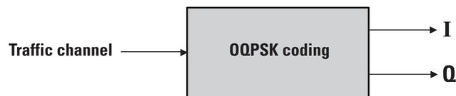
**Figure 2. IS-95 reverse channel coding**
