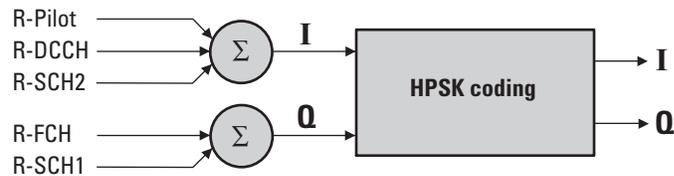
Figure 3. cdma2000 reverse channel coding
