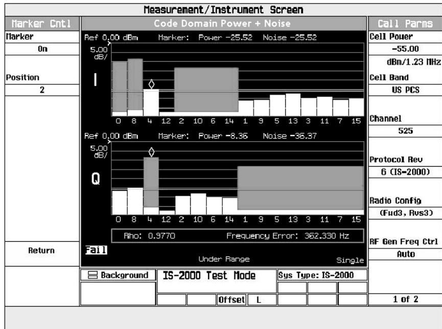
Figure 5. cdma2000 multi-coded code domain power display
