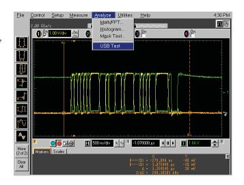
Figure 2. D+ and D- data signals are automatically bracketed by the Agilent Infinium Series USB Test Option.
