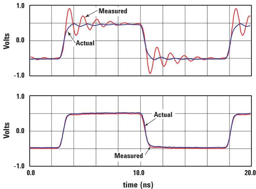
Figure 9. Measurements taken on a 66 MHz/500-ps clock.
