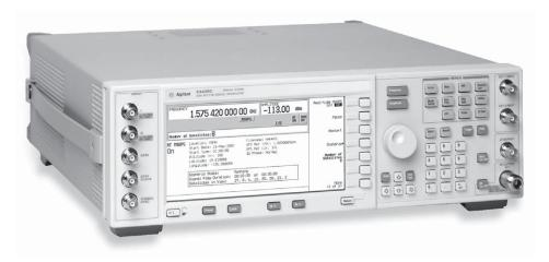
The Global Positioning System (GPS) personality (Option 409) for the E4438C ESG or E8267D PSG vector signal generator simulates a multi-satellite GPS signal for GPS receiver testing. This firmware option provides the capability to verify functionality of embedded GPS chips in mobile consumer products such as cellular phones and handheld receivers.
