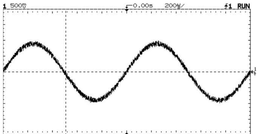
Figure 6. Measuring rms on a noisy sine wave
