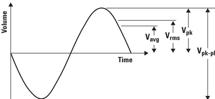
Figure 1. Common voltage parameters
