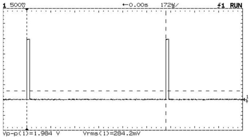
Figure 5. Measuring rms on a low-duty-cycle pulse train
