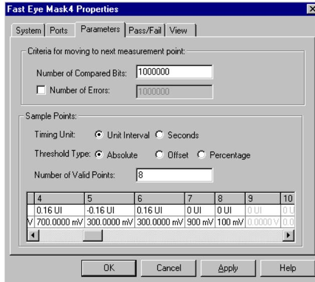
In the figure above, two measurement points have been added at 0 UI as absolute voltages.
