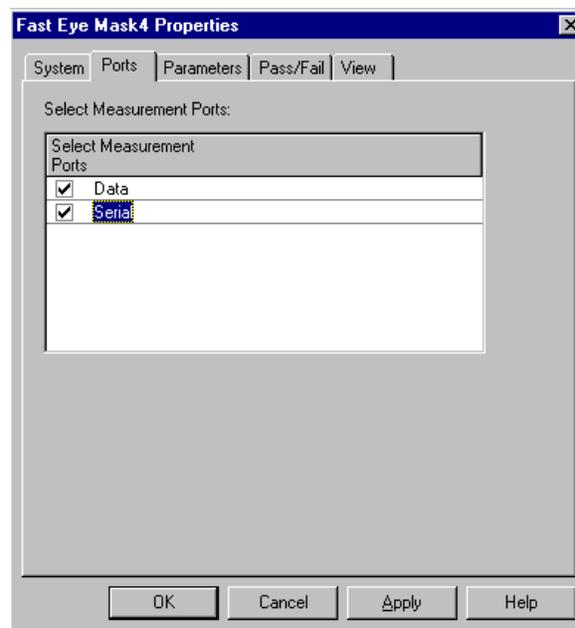
The *Ports* page lists all the output ports of the device under test, as defined in the loaded setting. In case of two systems, this is the setting loaded on the analyzing system. By default, all these ports are enabled and will be measured.
