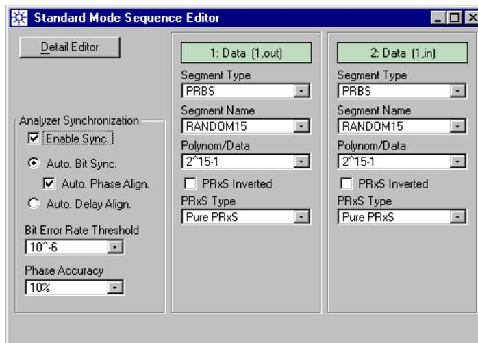
*Automatic Bit Synchronization* with *Automatic Phase Alignment* ensures that the analyzer will position its sampling point automatically at the optimum, no matter what the total signal delay is.
