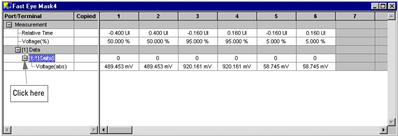
**Bit Error Rate** You can display the bit error rate calculated from *All Errors* (default), *1s Errors*, or *0s Errors*.
