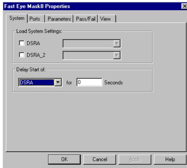
If you have already loaded a setting with the *Agilent 81250 User Software*, the name of this setting will be displayed, and it will be used by default.
