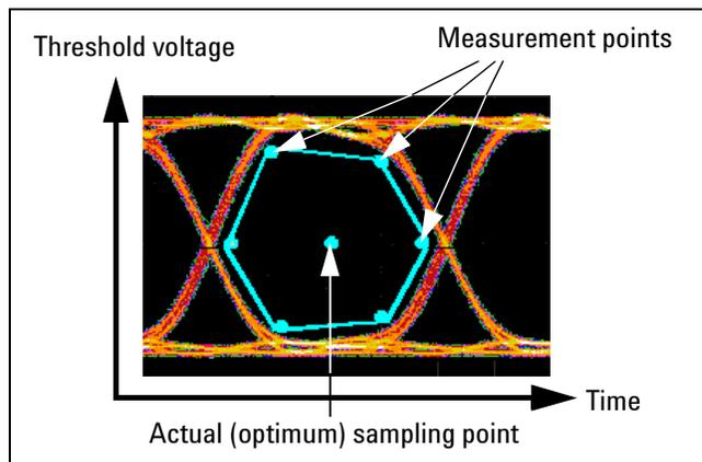
Up to 32 measurement points can be specified, each defined by a sampling time relative to the actual sampling point (which can be the optimum sampling point) and a threshold voltage (which can be fixed or adaptive). In practice, six measurement points will often suffice. Six measurement points are preset by default.
