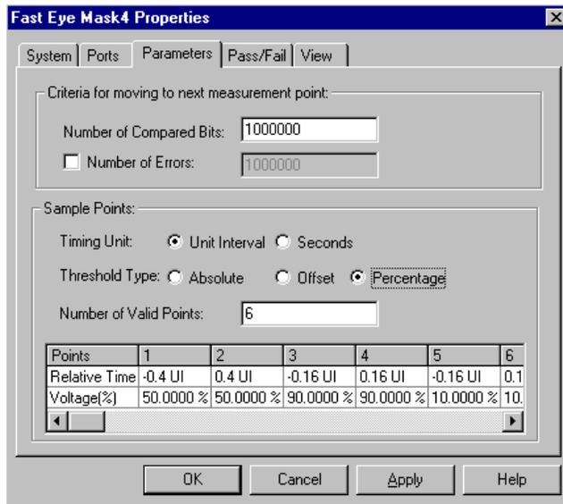
**TIP** If your analyzers have been configured to use different threshold levels, you should use the options *Offset* or *Percentage*. These options consider the settings of the individual analyzers.
