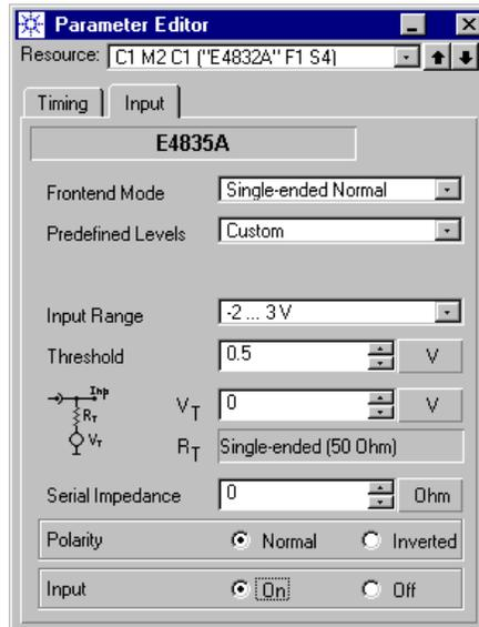
Measuring eye openings requires an analyzer threshold voltage. The fast eye mask measurement can therefore not be performed in differential mode.
