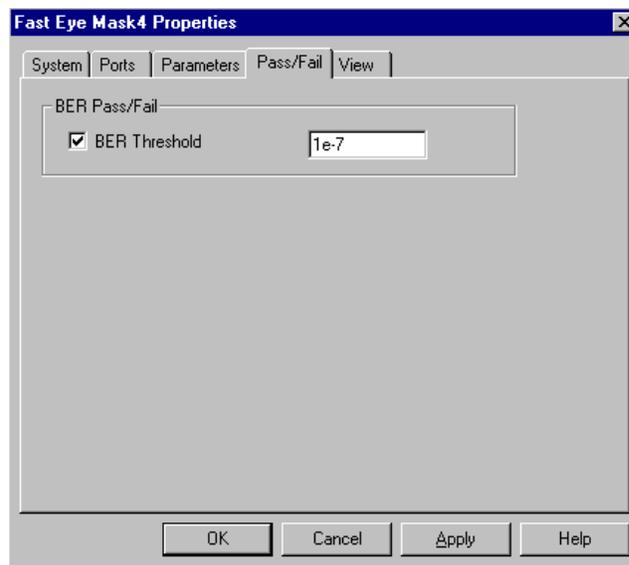
The minimum useful threshold is determined by the *Number of Compared Bits* (see “*How to Set the Criteria for Moving to the Next Point*” on page 31).
