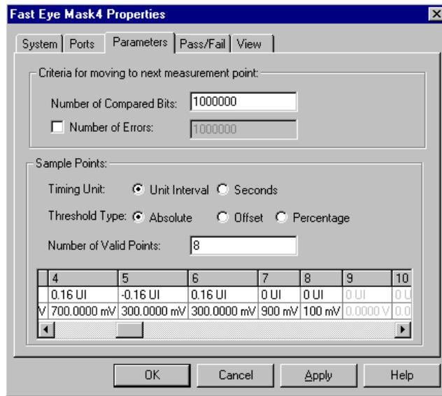
In this example, we will measure the bit error rate at the actual analyzer sampling point, using threshold voltages of 0.1 and 0.9 V.
