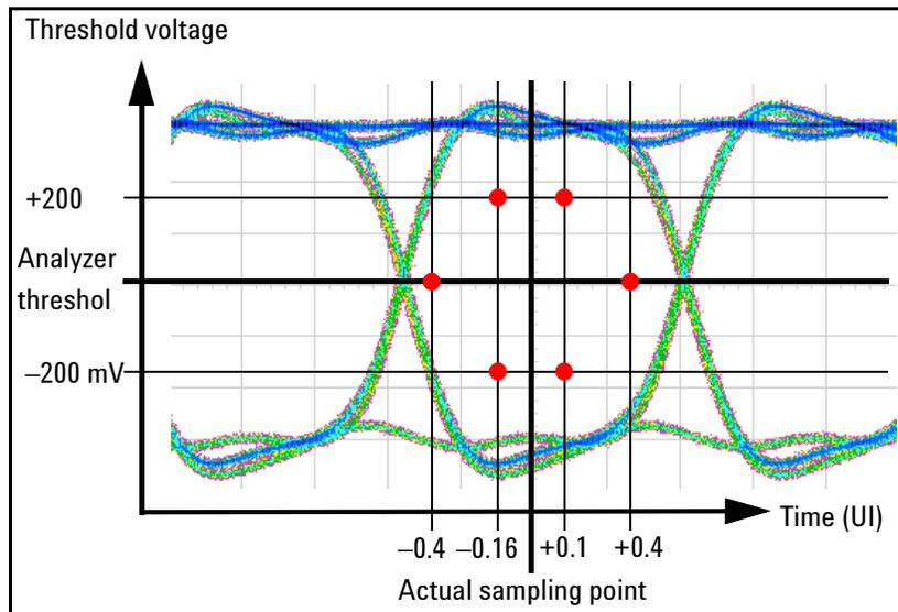
The relative time refers to the actual sampling point. In this example, where *Automatic Bit Synchronization* with *Automatic Phase Alignment* was set, this is the optimum sampling point. The time unit is UI (Unit Interval). One UI is the period of the current clock frequency. If the system clock frequency is 125 MHz, one UI is 8 ns.
