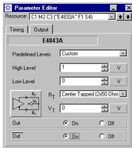
We use a voltage swing of 0 V (*Low Level*) to 1 V (*High Level*) in this example.
