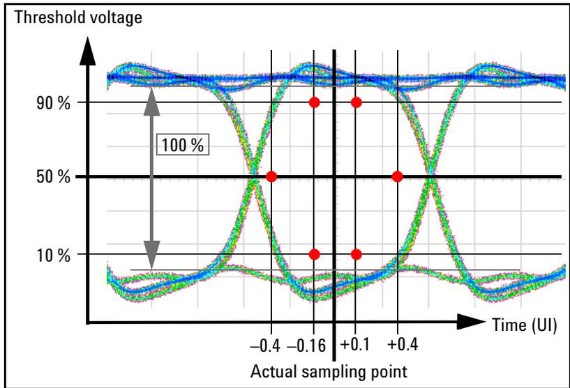
Depending on the quality and characteristics of the eye opening, the resulting 50 % threshold may deviate from the analyzer threshold defined in the loaded setting.
