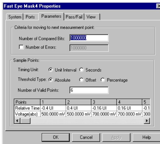
By default, the *Timing Unit* is *Unit Interval* (UI), the *Threshold Type* is *Absolute*. Six measurement points are preset.
