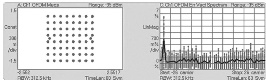
Figure 12: OFDM EVM versus frequency with spur
