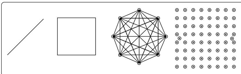
Figure 7: Example 802.11g modulation types (right to left: BPSK, QPSK, 8PSK, and 64QAM)
