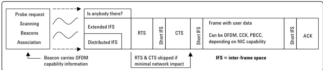
Figure 5: Example 802.11g packet under AP control
