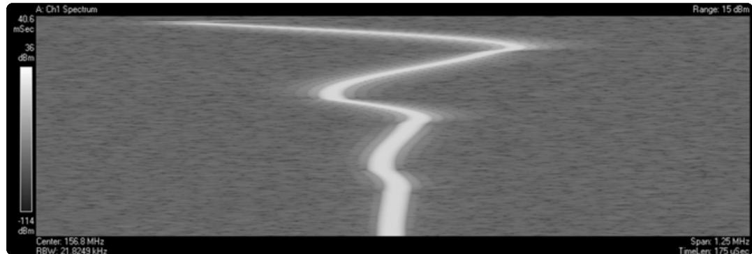
Figure 9: Spectrogram display of a VCO turn-on transient
