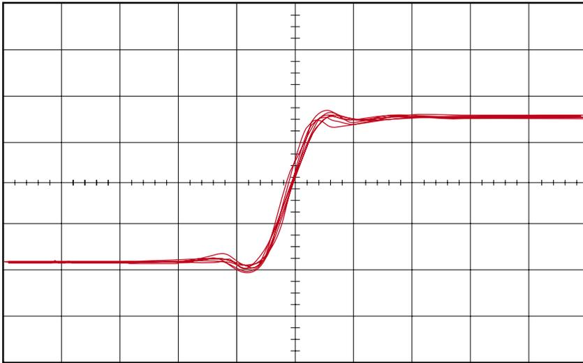
**Figure 5. Waveform wobble due to sampling alias error**
