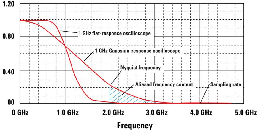
Figure 1. One GHz bandwidth oscilloscope frequency responses
