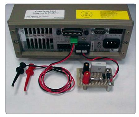
Figure 2. Example of an external protection network and DVM leads
