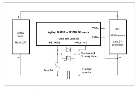
Figure 1. Recommended test set-up
