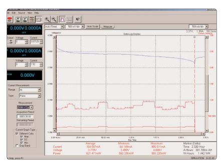
**Figure 3.** 14565B Data log mode displaying a battery run-down test
