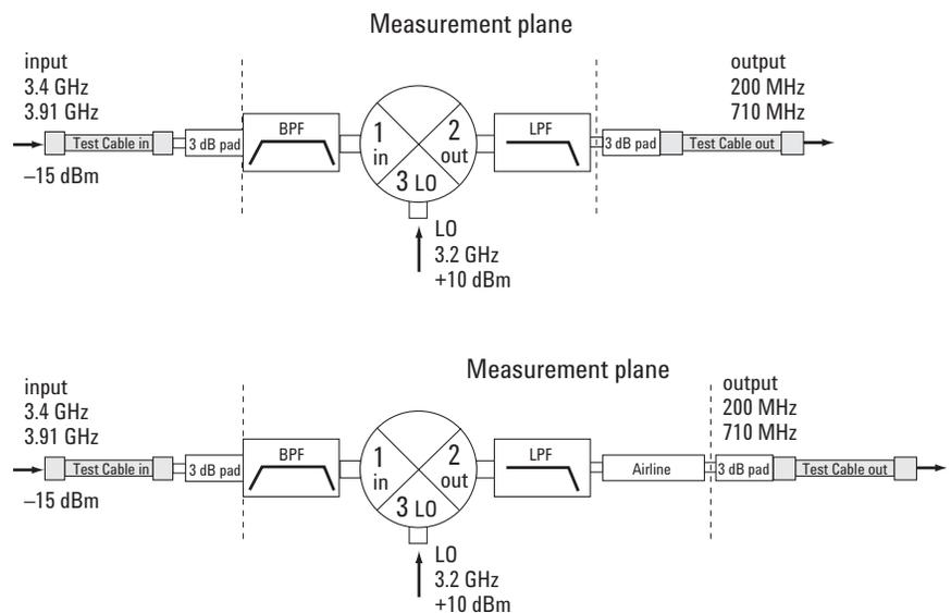
Figure 9. Converter configuration for airline delta comparison.
