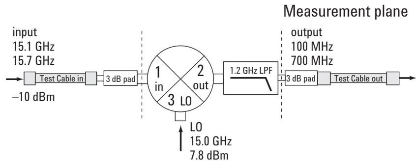
Figure 1. Example of a mixer-under-test configuration.
