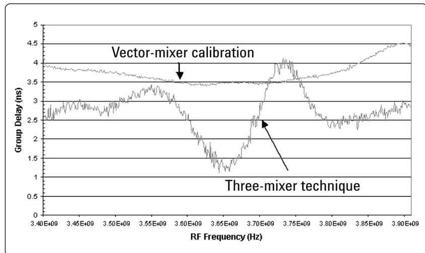
Figure 12. Measurement comparison of group delay techniques.
