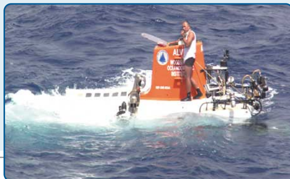
Figure 3 (Below). The 23-foot Alvin submersible, with two scientists and a pilot on board, typically conducts 10 hour dives.
