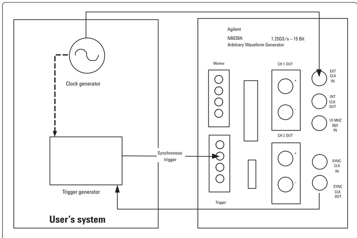
Figure 4 Synchronous trigger usage example
