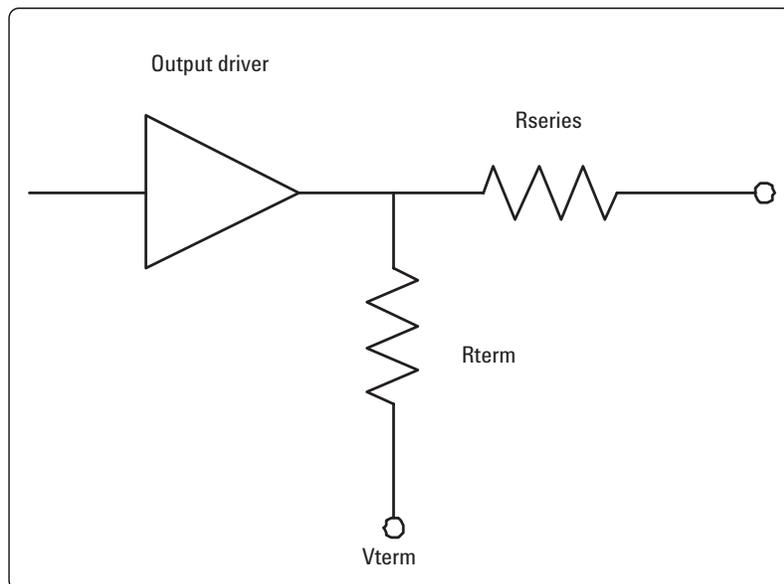
Figure 3. Generic output driver diagram
