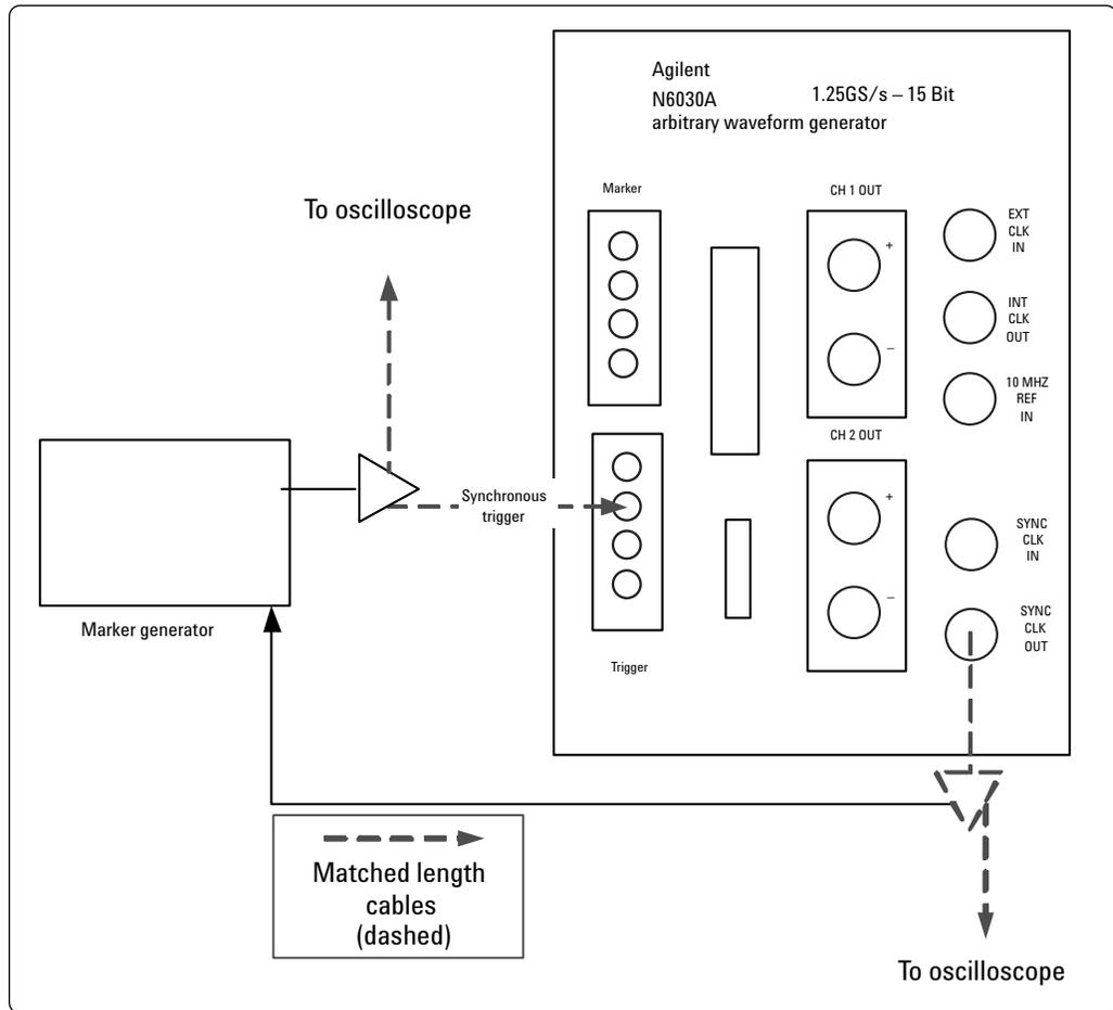
Figure 2. Trigger input timing measurement
