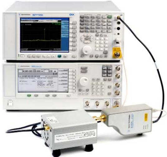
Figure 10. Millimeter wave source module works with the Agilent M1970 Smart Mixer to create a stimulus-response test system.
