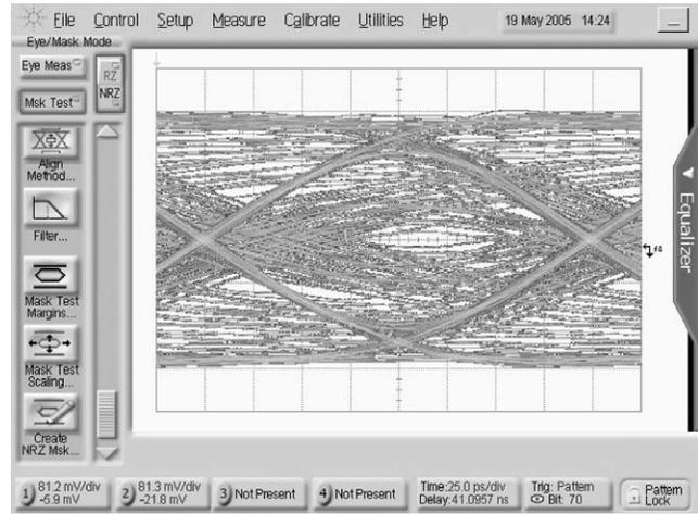
Figure 7: The received and equalized eye diagrams.
