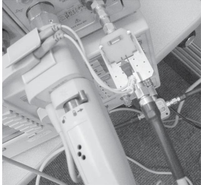
**Figure 3: The E2655B Deskew and Performance Verification fixture allows for easy probe calibration with the 86100 DCA**
