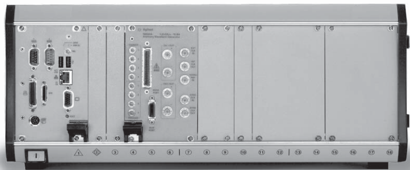
Figure 12. Agilent N6033A AWG with controller in CompactPCI chassis
