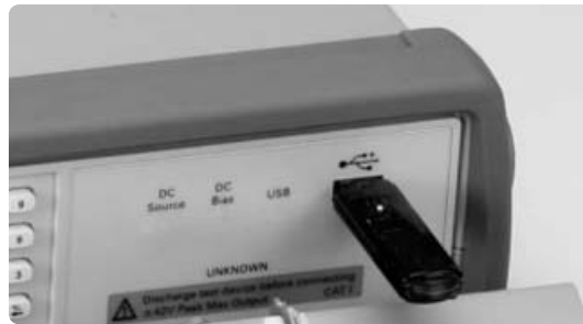
Figure 6. A USB memory device can be used to remotely and easily save set up states, data or graphs.
