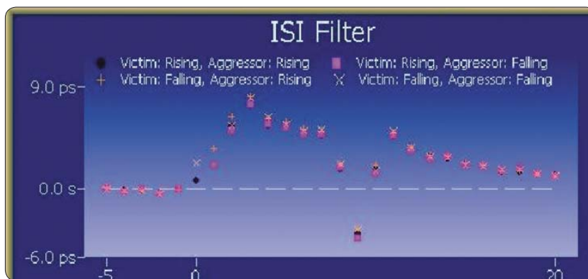
Figure 3. This ISI filter graph shows how the transitions surrounding each bit affect that bit's data-dependent jitter.
