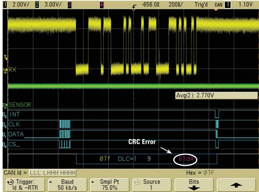
**Figure 4: Random errors observed in CAN decode while triggering on data frame ID: 07F<sub>HEX</sub>**
