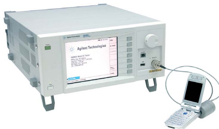
Figure 3: N9360A test set connected to a mobile phone
