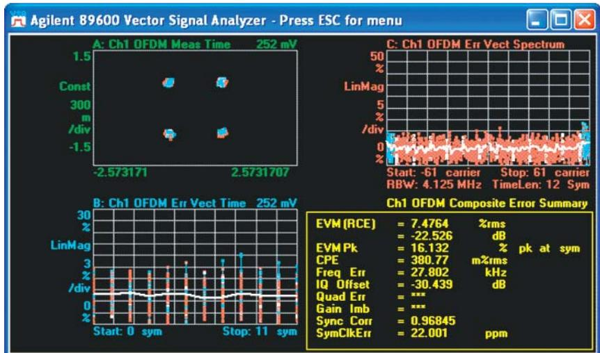
Figure 1. Option BHB MB-OFDM ultra-wideband modulation analysis offers detailed error analysis down to the individual carrier (Trace C, upper right) or individual symbol (Trace B, lower left). For an overall view, composite errors are shown in the table (Trace D, lower right).
