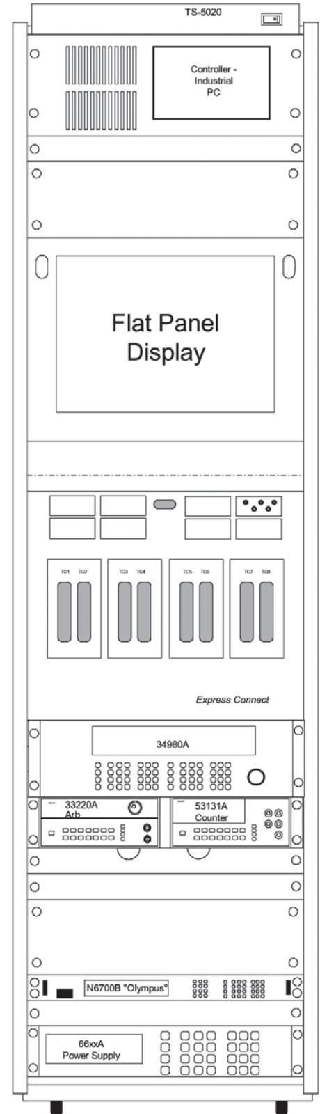
Figure 3. Agilent TS-5020 automotive functional test system
