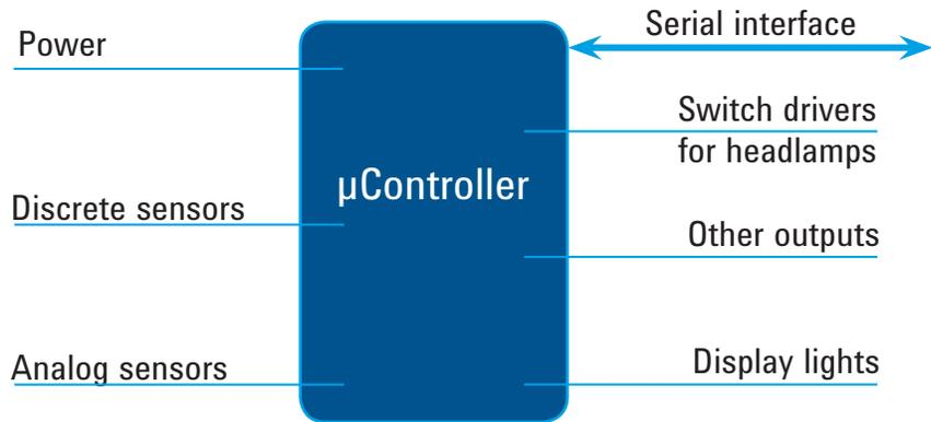
Figure 5. Example of serial interface for an electronic control module (ECM).
