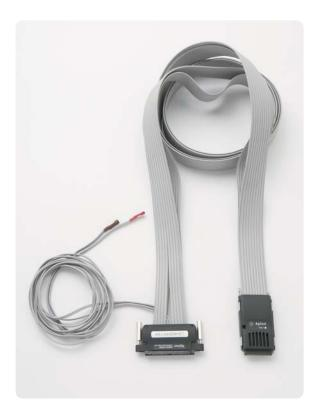
Figure 10. N4241A/2A/3A mid-bus probe
