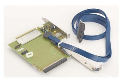
Figure 16. N5315A slot interposer probe
