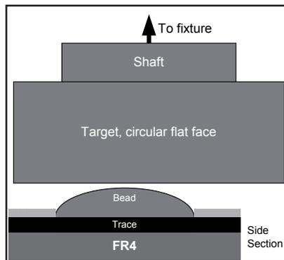
Figure 2: Side view of bead probe and target
