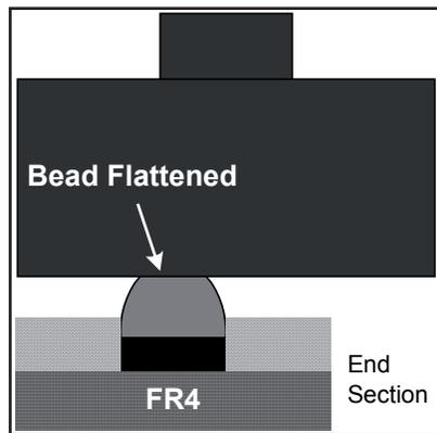
Figure 4: A bead probe flattens when contacted.
