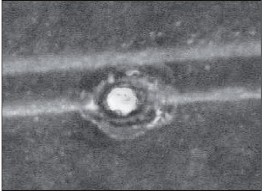
*Figure 13: Topside photo of a probed bead. Note flattened surface.*
