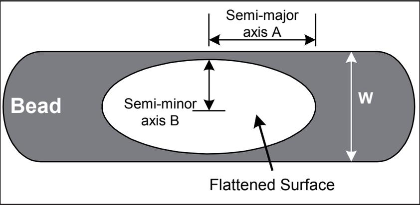
Figure 5: Top view of a flattened bead.
