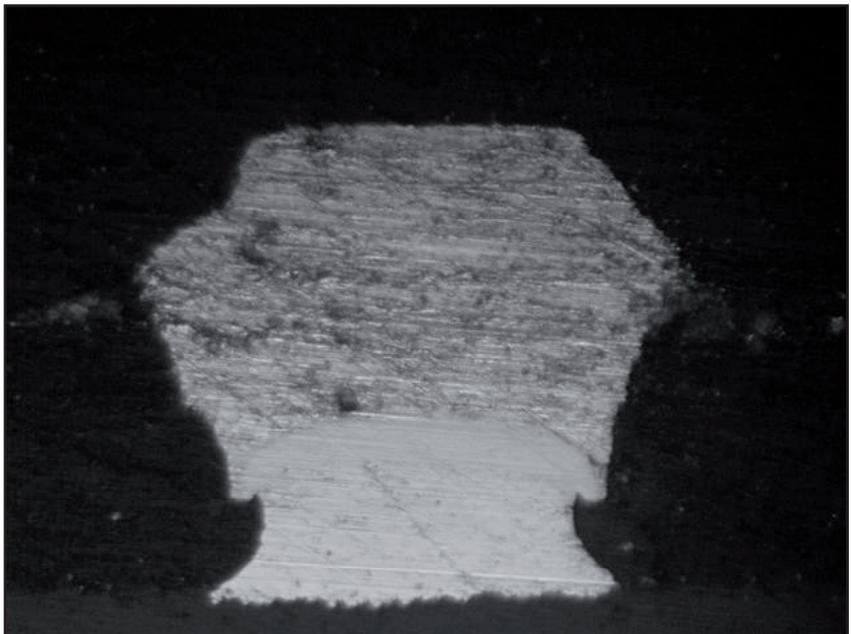
*Figure 14: Cross section of a flattened bead.*
