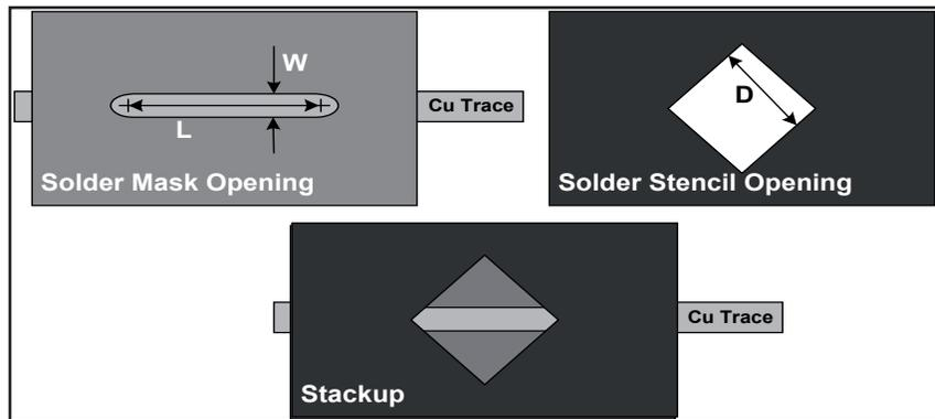
Figure 3: Board, solder mask and solder stencil layer stack up for a bead probe.
