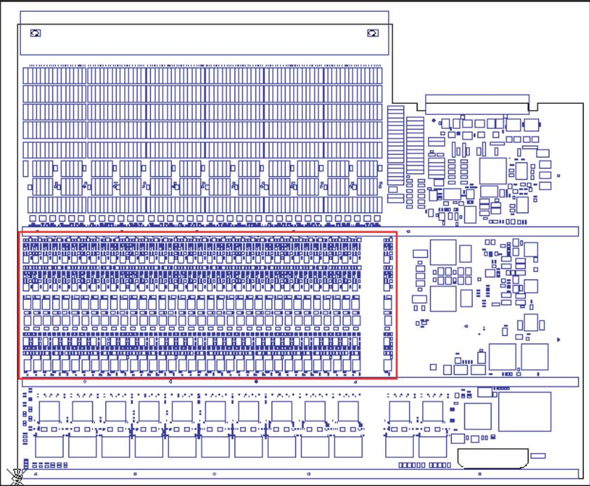
Figure 15 – PCA with bead probes
