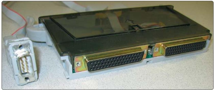
Figure 1: Y1131A hardware: a custom terminal block.
