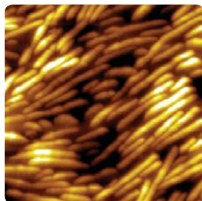
Figure 4. Images of temperature-induced phase transition of polypropylene. Scan sizes: 2 \mu\text{m} x 2 \mu\text{m} .
