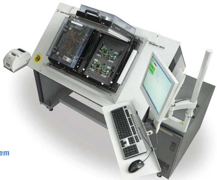
The Agilent *Medalist i3070* In-Circuit Test system combines all the features of a state-of-the-art Agilent *Medalist 3070* with the advanced architecture and streamlined usability of the Agilent *Medalist i5000*. You get an intuitive point-and-click interface, automated test debug and optimization tools, and a host of other features to accelerate every aspect of test programming and deployment.
