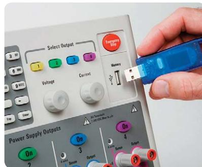
Figure 12. The N6705's front panel USB port.
