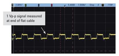
Figure 4. Low signal loss.
