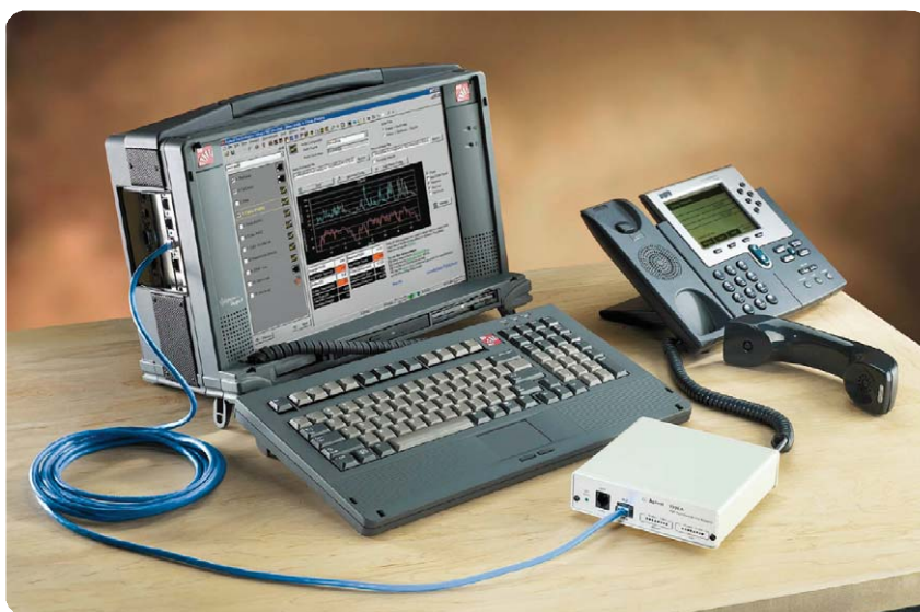
VQT analog interface card in a ruggedized PC with the Agilent Phone Adapter
