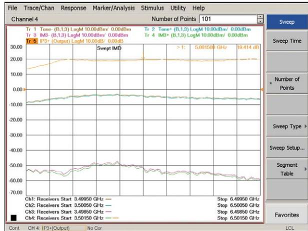
**Figure 4. PNA-X example of a swept-frequency IMD measurement**
