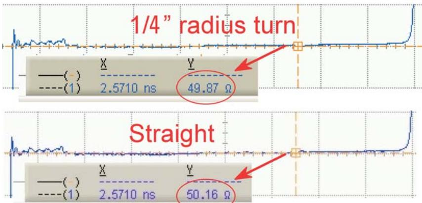
Less than 1% impedance change for bent cable
