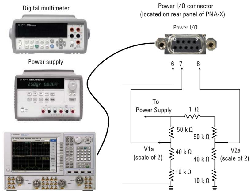
**Figure 10.** An example of the setup used to calibrate the analog inputs of the PNA-X. In this example, connections made to pins 7 (AI1) and 8 (AI2) are also made to the digital multimeter for readings comparison. Pin 6 is ground. Resistive circuit shown is the same as that of Figure 6, and output with a scale of 2 is used in this example.
