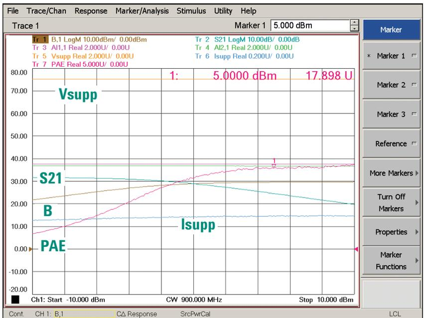
Figure 3. Measurements made over power sweep, including PAE.
