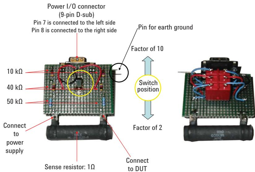
**Figure 7.** Actual realization of the sensing circuit shown in Figure 6. Left: top view, right: bottom view.
