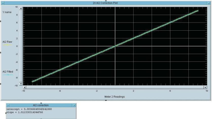
Figure 12. Example of data gathered for AI2 using resistive circuit shown in Figures 6 and 7 (with a scale of 2).
