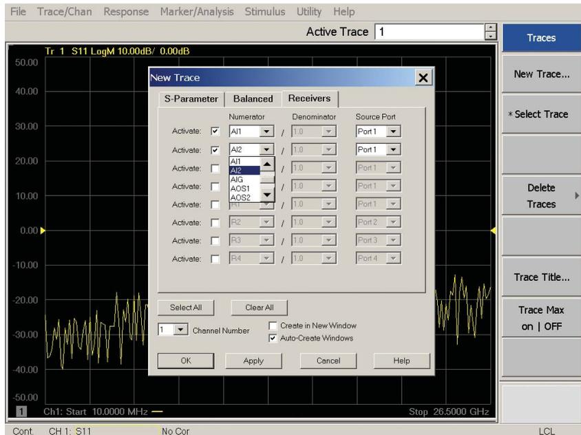
**Figure 8.** Simple steps to add AI1 and AI2 traces onto the PNA-X display. Other analog measurements available include AIG (analog input ground), AOS1 and AOS2 (analog output sense 1 and 2, respectively).
