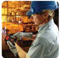
Regular maintenance with an accurate, dependable DMM ensures early detection of harmonics in the AC supply. One of the quickest ways to detect and gauge the percentage of distortion due to harmonics is to measure the harmonic ratio of the incoming AC voltage.
