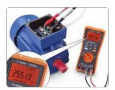
to quickly determine if the problem is contributed by unwanted high frequency components generated by the VFD. The Agilent U1270 Series handheld DMMs offer a 1 kHz low pass filter to provide accurate VFD output measurement. This function eliminates unwanted high frequency noise signals and components generated by the VFD. Therefore, a technician would be able to reduce troubleshooting time and ultimately reduce system downtime.
