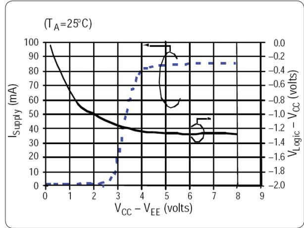
Figure 5. Typical supply current &  $V_{Logic}$  vs. supply voltage
