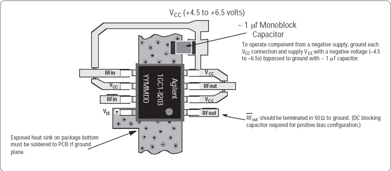
Figure 3. Assembly diagram (Single-supply, positive-bias configuration shown)
