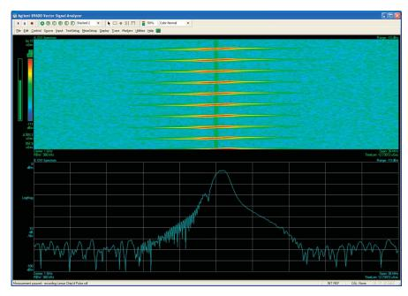
Figure 5. Pulsed RF linear chirp with spectrogram and frequency spectrum
