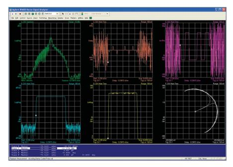
Figure 4. Barker coded pulsed RF showing frequency, delay, phase, time (log), time (linear), and  $I/\Omega$
