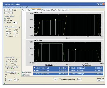
Figure 3. PAS system shows the RADAR mode changes with PRI vs time and PW vs time
