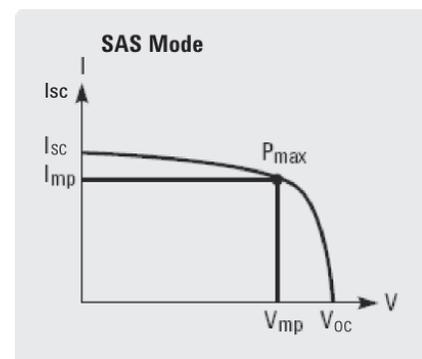
Figure 1: Power supply output characteristic in SAS mode
