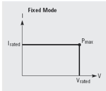
Figure 2: Power supply output characteristic in Fixed mode
