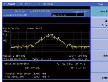
Figure 2 Channel bandwidth measurement
