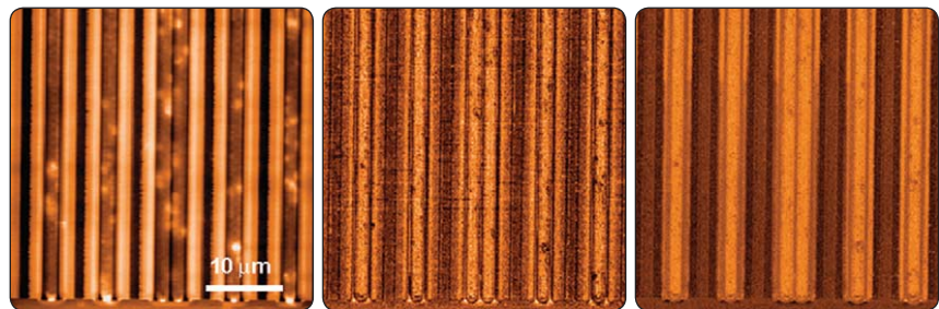
Topography (left) capacitance (middle) and dC/dV (right) images of a doped SiGe device acquired with a scanning microwave microscope. Both capacitance and dC/dV images showed some dopant structure not seen in the topography. (W. Han)
