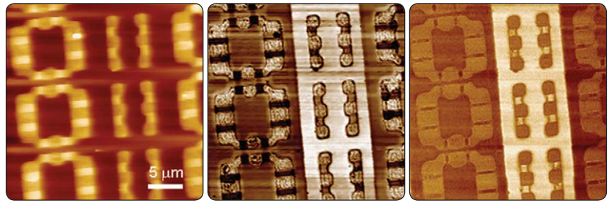
Topography (left), capacitance (middle) and dC/dV (right) images of a SRAM chip acquired with a scanning microwave microscope. The underneath n-type (bright) and p-type doped structure are clearly identified in both capacitance and dC/dV images. (W. Han)
