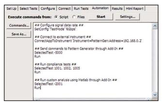
Figure 7. Remote Programming script in the Automation tab.
