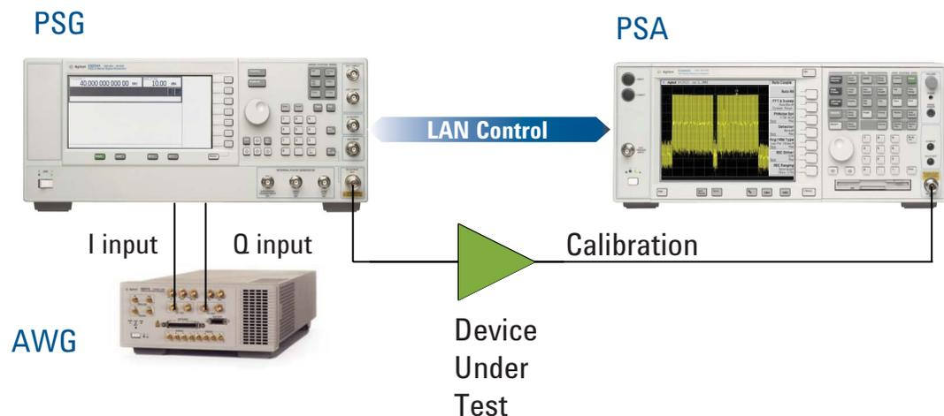
Figure 5. Digital NPR measurement system setup
