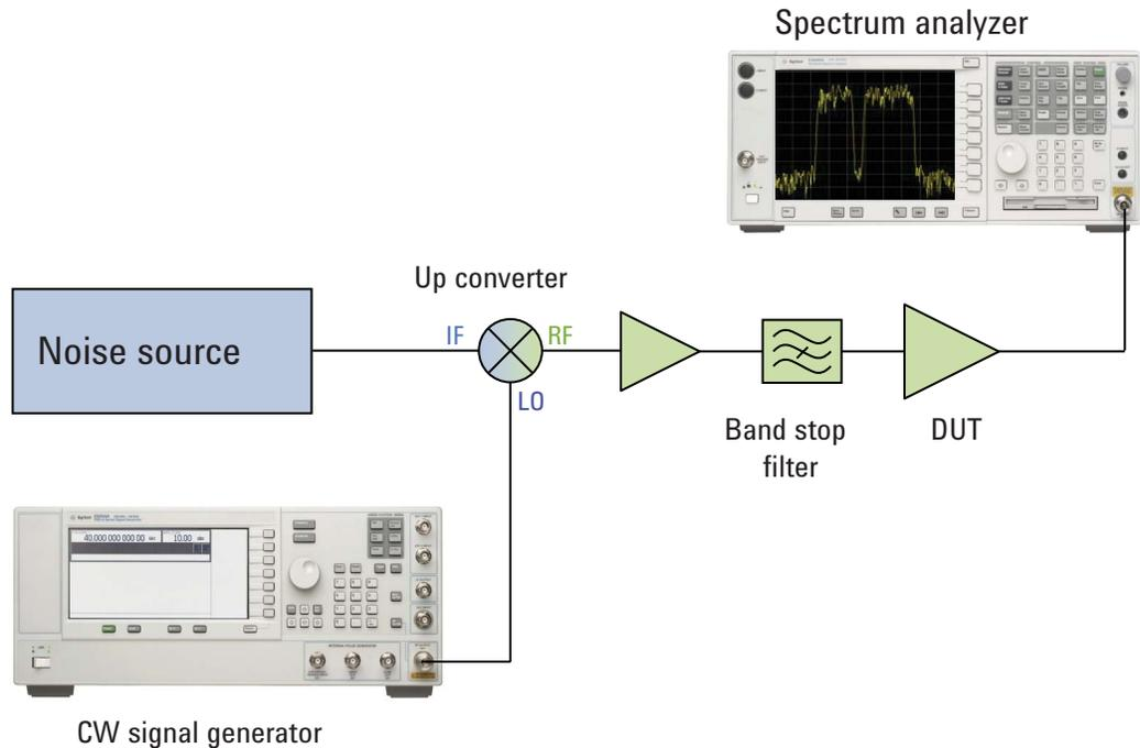
Figure 3. Traditional (analog) NPR test setup
