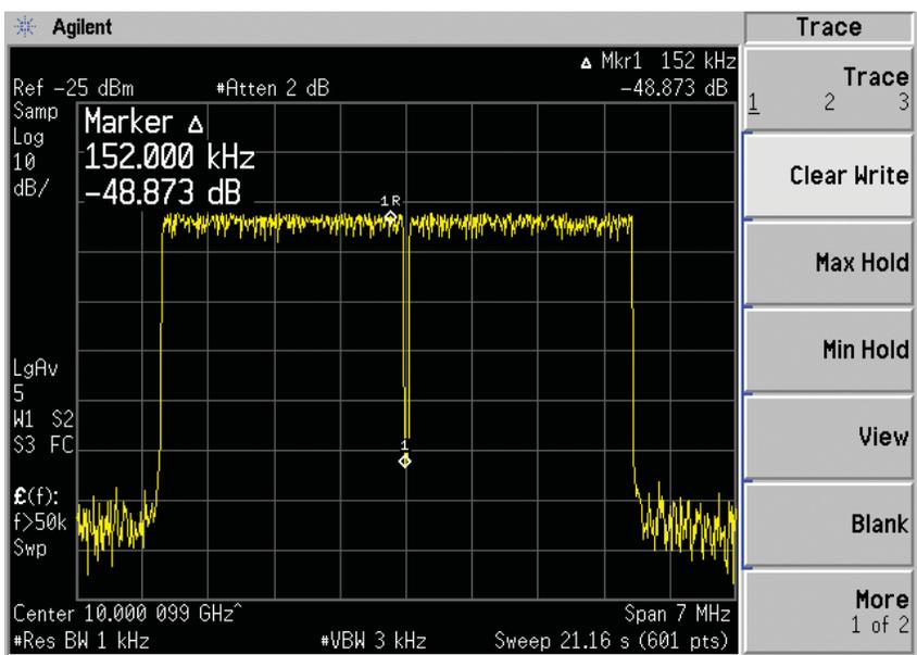
Figure 6. Digital stimulus spectrum measured in line mode
