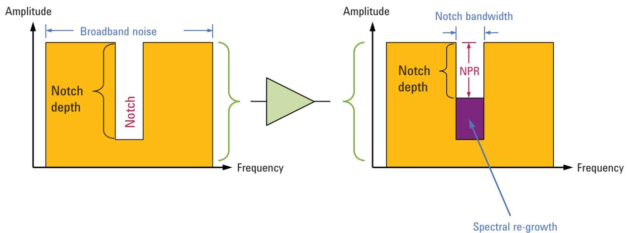
Figure 2. NPR stimulus before and after the device under test
