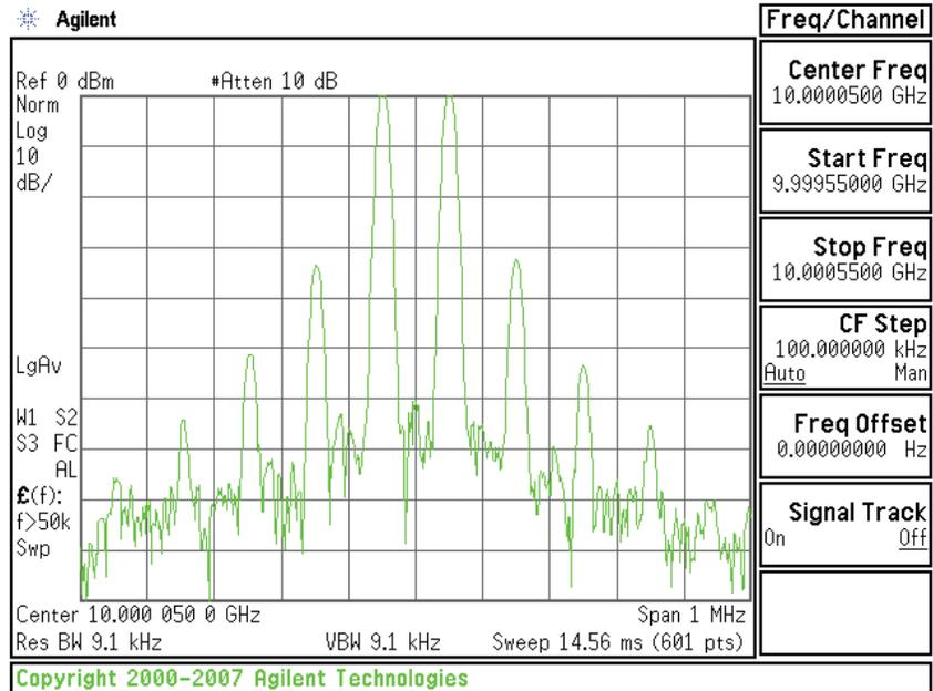
Figure 1. Multiple output distortion tones in a non-linear system
