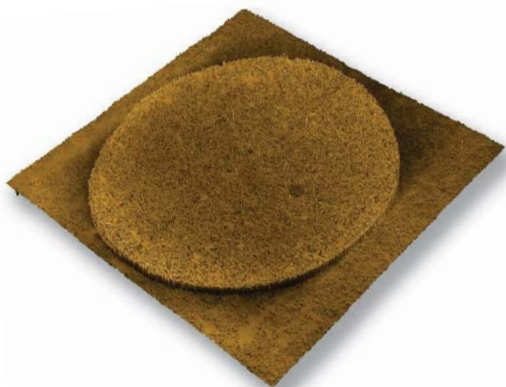
3D AFM image of an Agilent DNA microarray.
