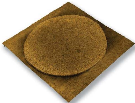
Figure 2. 70 x 70 microns 3D AFM image of the DNA microarray shows a single oligonucleotide probe element surrounded by the silanized glass substrate. The difference in height between the probe area and the bare substrate is clearly visible.
