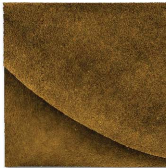
Figure 3. 15 x 15 microns 3D AFM image of the DNA microarray shows the contrast between a probe element and the surrounding silanized glass substrate (lower left).
