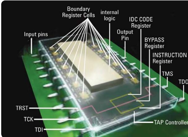
Figure 1. A boundary scan device
