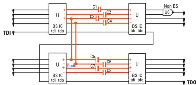
Figure 9. Agilent *Medalist i3070* Bus wire test on 1149.6 DC/AC differential signals.
