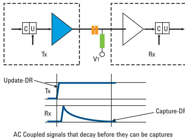
Figure 7. Differential Signal with AC coupling.
