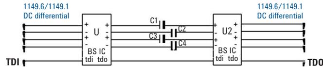
Figure 11. Agilent *Medalist* i3070 connect test on 1149.6/1149.1 DC differential only.
