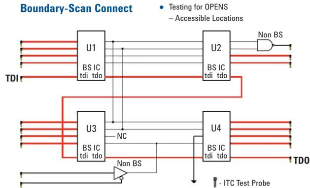
Figure 6. Connect Test checks the connections of each device in a chain.
