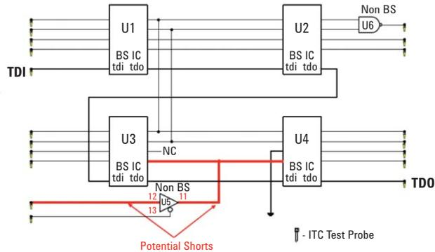
Figure 4. Agilent’s Powered Shorts test checks for shorts between boundary-scan nodes without test probe and any nearby non Boundary Scan node with test probes.
