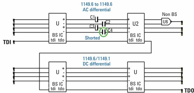
Figure 8. Agilent *Medalist i3070* interconnect test and shorted capacitor test on 1149.6 DC/AC differential signals.
