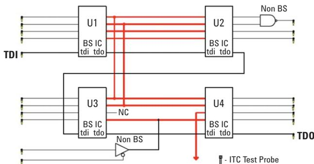
Figure 3. Interconnect Test checks connections for most shorts and some opens within the chain.
