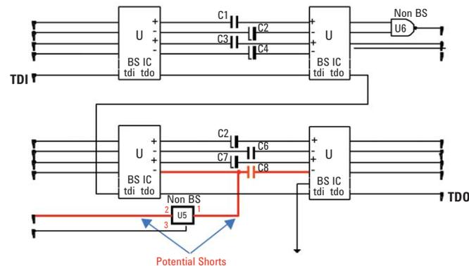
Figure 10. Agilent *Medalist i3070* Powered short test on 1149.6 DC/AC differential signals.
