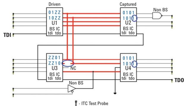
Figure 5. Bus Wire Test verifies connections on bussed nodes.
