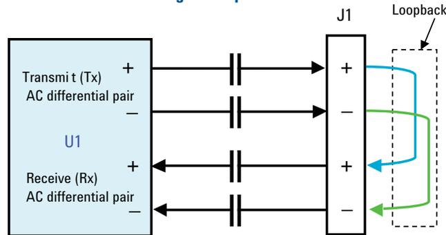
Figure 12. 1149.6 AC Differential Loopback testing
